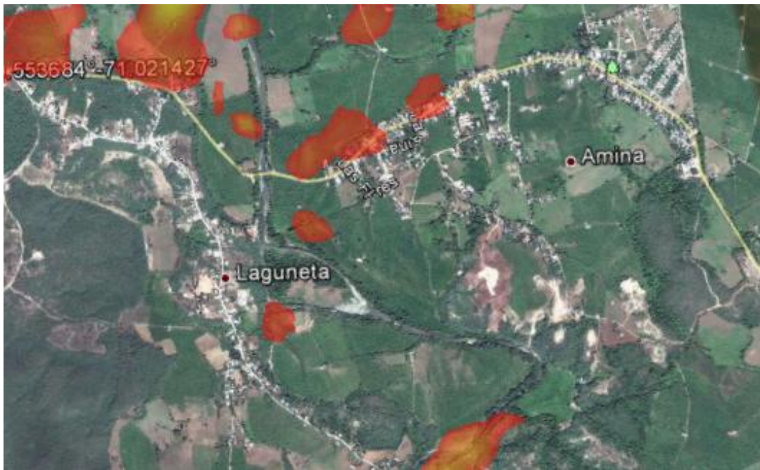
Figure 13. Flooding in the town of Amina during a 100-year 24-hour storm with the proposed dam and reservoir at 75% capacity
