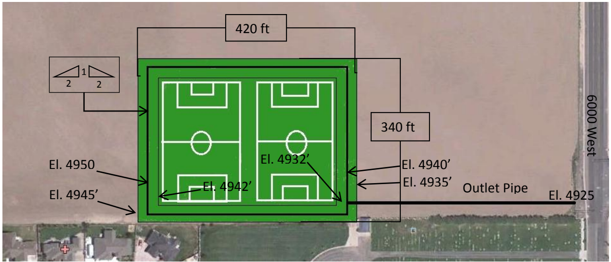
Figure 11. Detention basin measurements
