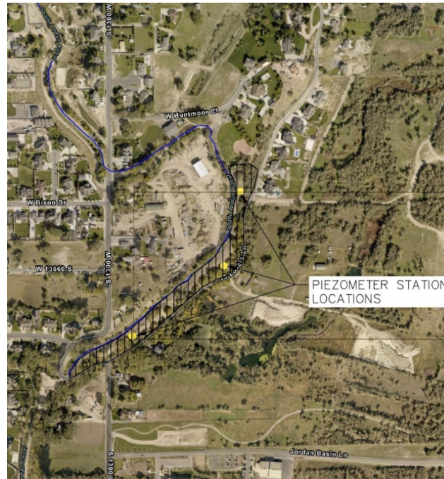
Figure 3. Locations for Piezometer Stations
