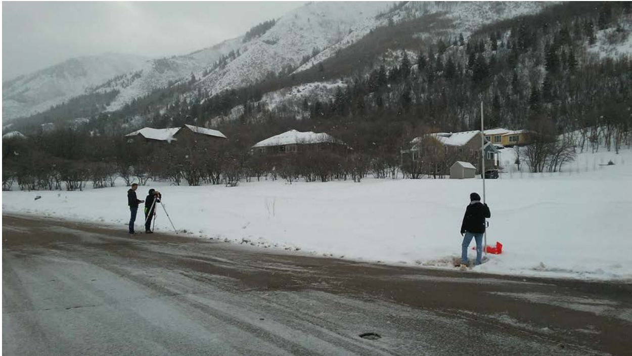
Figure 9: Measuring longitudinal slopes for channel design inputs.
