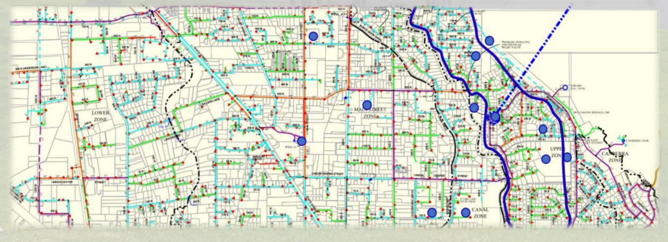
In order to resolve the loop issue, we found it was necessary to extend the connection point, of the 0.5 MG and 1 MG tanks to the main line on Center street from 700 E and 400 E. This provided an access point for the water where it wouldn't be immediately transferred to the upper zones. The image below shows the extension of the 18" pipe from 700 E to 400 E.
