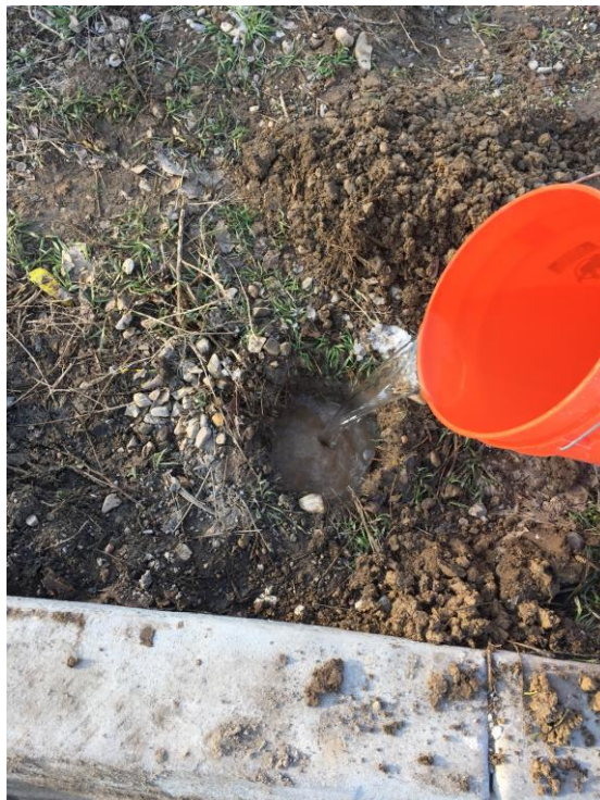
Figure 4: Filling up the test hole with water
