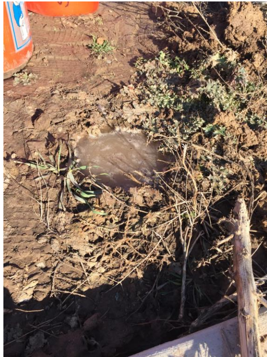
Figure 5: Test hole filled with 12 in water
