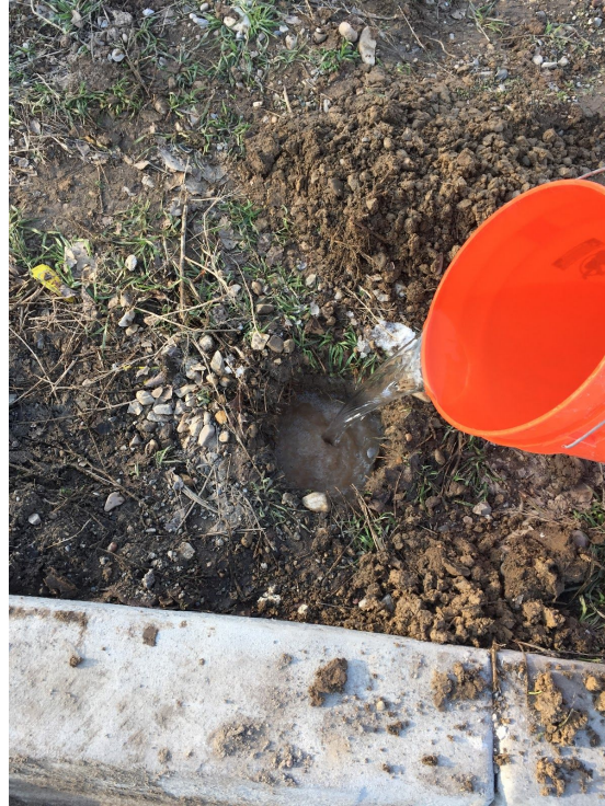
Figure 4. Filling up the test hole with water
