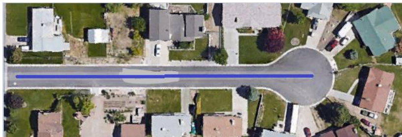
Figure 1 A common Riverton Cul-de-sac with the open ended water line illustrated in blue.
