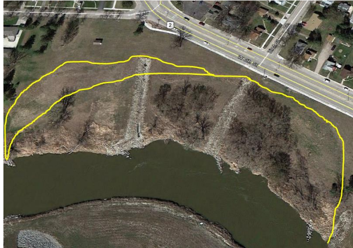
Figure 2: Limits of slope failure
